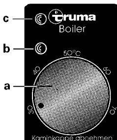
a = Rotary control knob On/Off and temperature control
